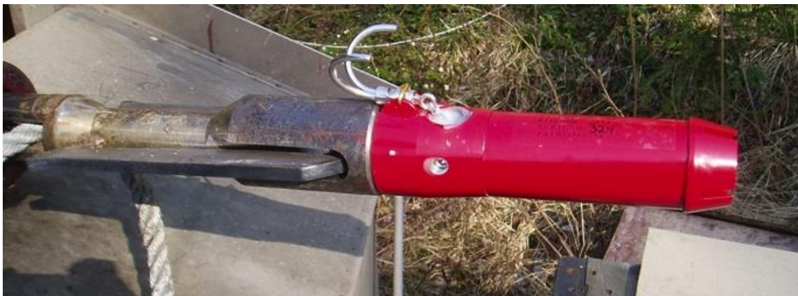
Fig. 27. Whale Grenade-99 with the triggerhook. (From test shooting of whale grenades). Photo: EO Øen
