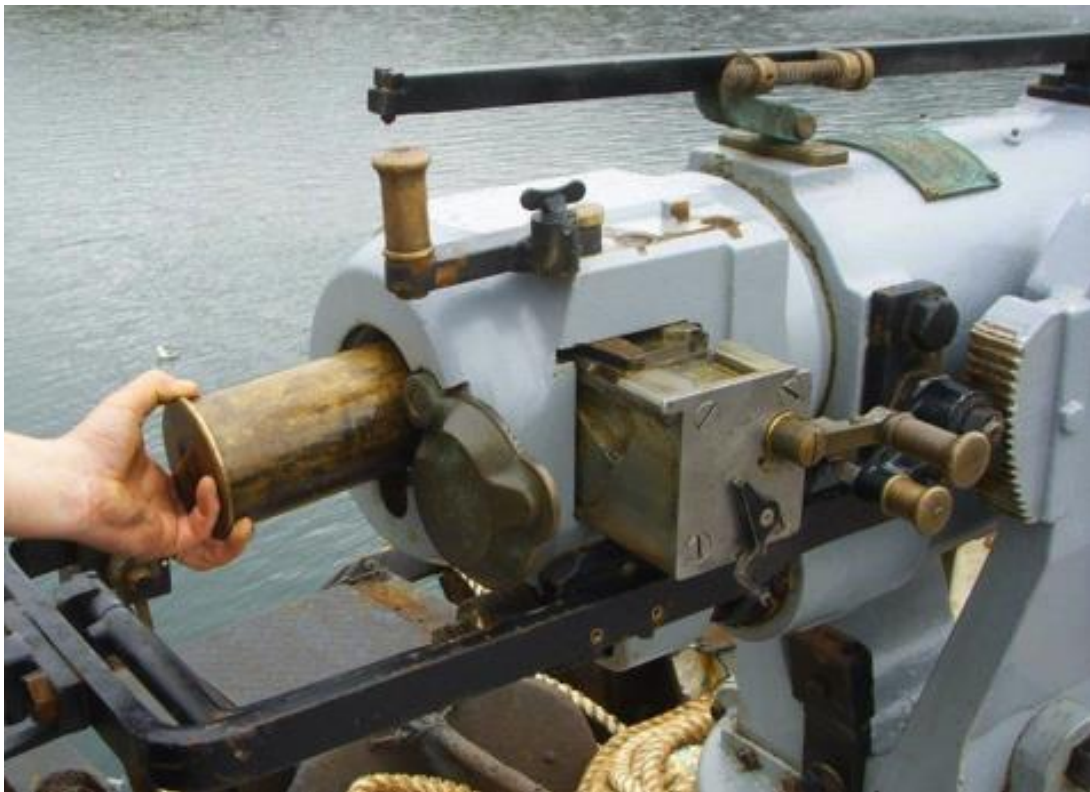
Fig. 16. Loading of 90 mm Kongsberg harpoon gun.
