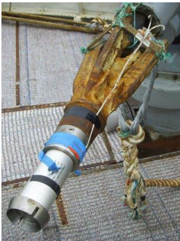
Fig. 18. 90 mm Kongsberg whaling gun with a harpoon and modified Whale Grenade-99 used for large whales. The trigger hook is fastened on the serving wire. Photo: EO Øen
