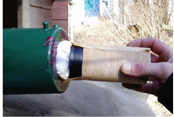
Figs. 20 and 21. Loading of 60 mm Henriksen whaling gun. (From test shooting of whale grenades) Photo: EO Øen
