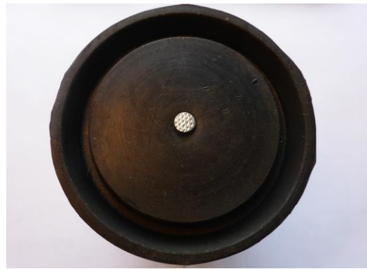
Fig. 14 and 15. Wadding and rubber washer for 90 mm Kongsberg harpoon gun. The rubber washer with sloping walls to the right.
