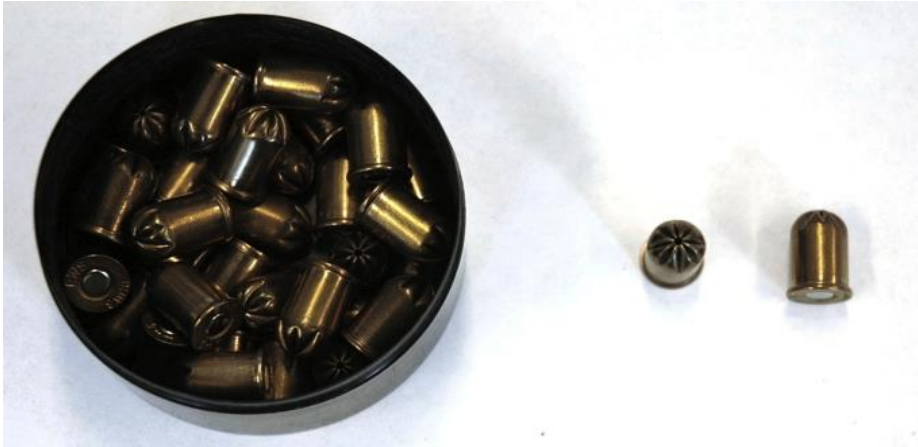
Fig. 8. Example of primers/firing cartridges for a 50 mm Kongsberg whaling gun. Photo: Nette Levermann
