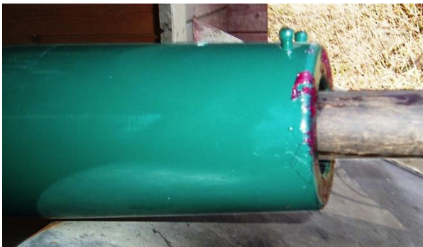
Fig. 22. Gunpowder bag is slid in to the bottom of the barrel with the charge stick. Photo: EO Øen
