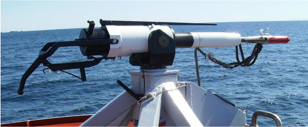
Fig. 2. 50 mm Kongsberg whaling gun with harpoon and Whale Grenade-99. Photo: Björgvin Guðmundsson
