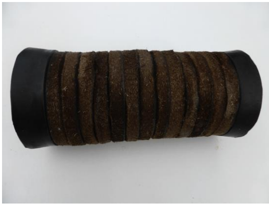
Fig. 14 and 15. Wadding and rubber washer for 90 mm Kongsberg harpoon gun. The rubber washer with sloping walls to the right.
