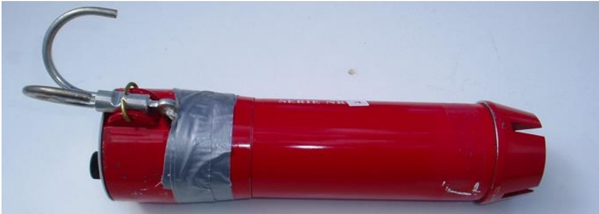
Fig. 29. Whale Grenade-99 where the loose trigger string is layed back in the plastic cup and taped fast.
