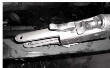
Fig. 24. Remington firing mechanism of a 60 mm Henriksen whaling gun. Photo: EO Øen
