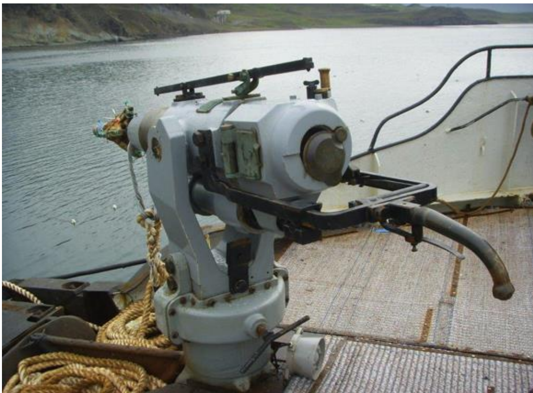
Fig. 11. Ready loaded 90 mm Kongsberg whaling gun.
