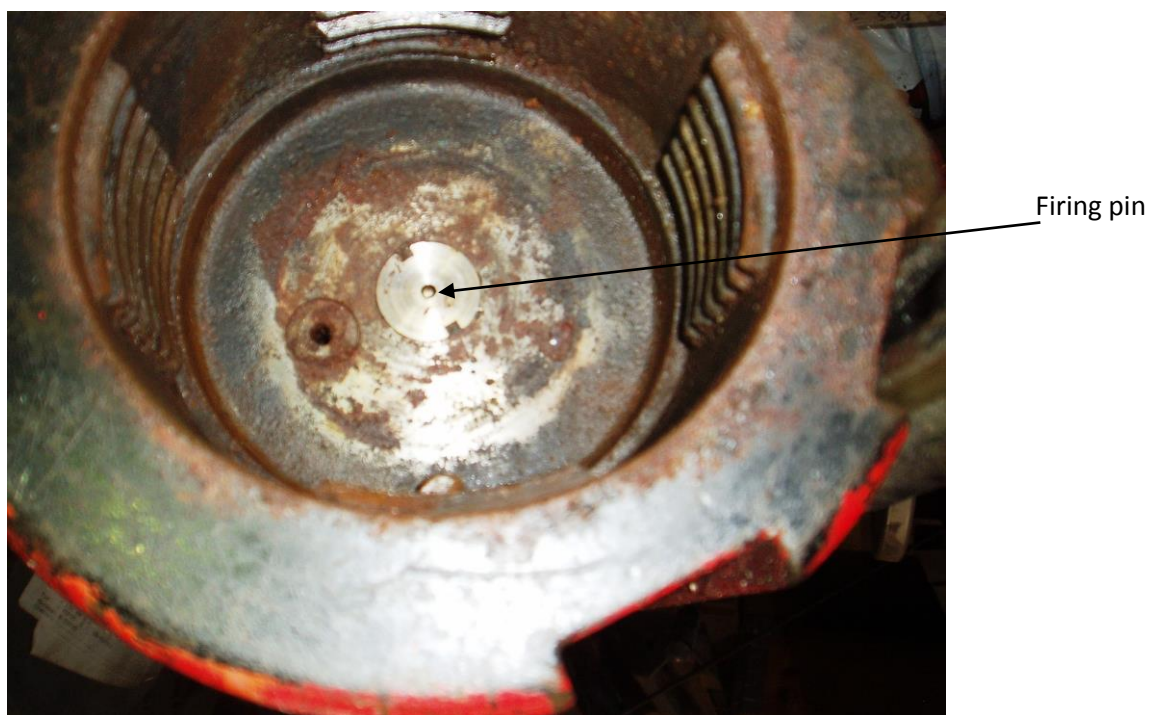
Fig. 5. Shock bottom in the breechblock of a 50 mm Kongsberg whaling gun. The firing pin is in the rear (secure) position. Photo: EO Øen
