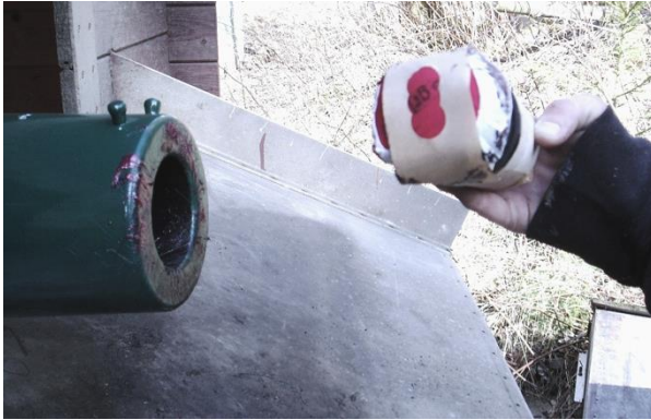
Figs. 20 and 21. Loading of 60 mm Henriksen whaling gun. (From test shooting of whale grenades) Photo: EO Øen
