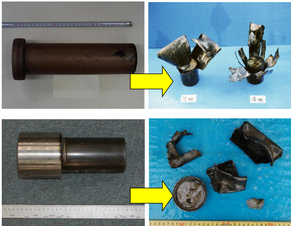
Fig. 1. (Upper) The traditional style harpoon head and shrapnel after explosion. A large shrapnel with a heavy weight was left in the whale body frequently. It sometimes cut harpoon line and caused “struck and lost”. (Lower) Improved harpoon head produces fewer and smaller shrapnel than the traditional one, which is expected to reduce possible struck and lost.
