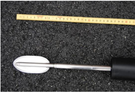
Fig. 21: New lance 6th version, blade details Photo: B. Hanusson
