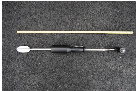
Fig. 20: New lance 6th version, sheath unlocked Photo: B. Hanusson
