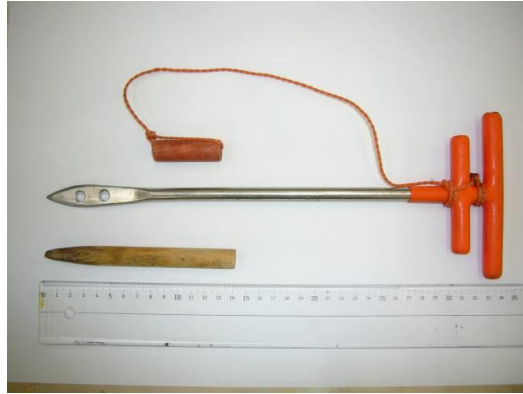
Fig. 5 Modified slaughtering knife and wooden plug (a piece attached to the knife is an indicator float when dropped into water)
