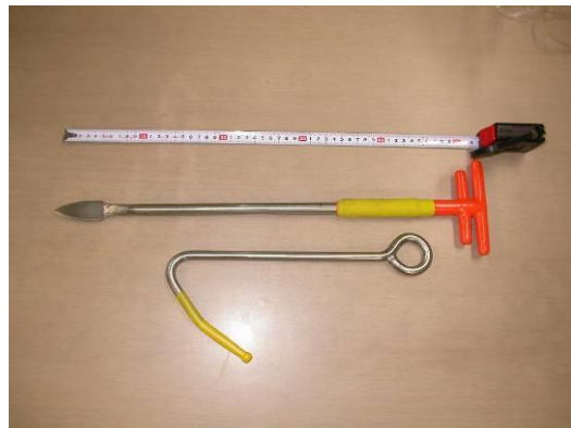
Fig. 3 Prototype of slaughtering knife (upper) and blowhole hook (lower) for Taiji fishery. Blowhole hook is now seldom used.
