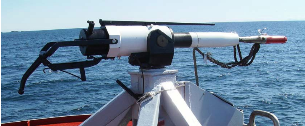
Fig. 1. 50 mm Kongsberg harpoon gun with harpoon and Whale Grenade- 99. Photo: Björgvin Gudmundsson
