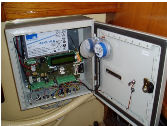
Fig. 3. The Blue Box (Control Box). The Automated Electronic Monitoring System for the minke whale hunt in Norway.
