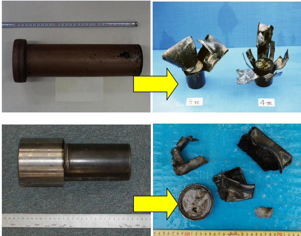
Figure 1. (Upper) The traditional style harpoon head and shrapnel after explosion. A large shrapnel with a heavy weight was left in the whale body frequently. It sometimes cut the harpoon line and caused “struck and lost”. (Lower) Improved harpoon head produces less and small sized shrapnel than the traditional one, which is expected to reduce possible “struck and lost”.
