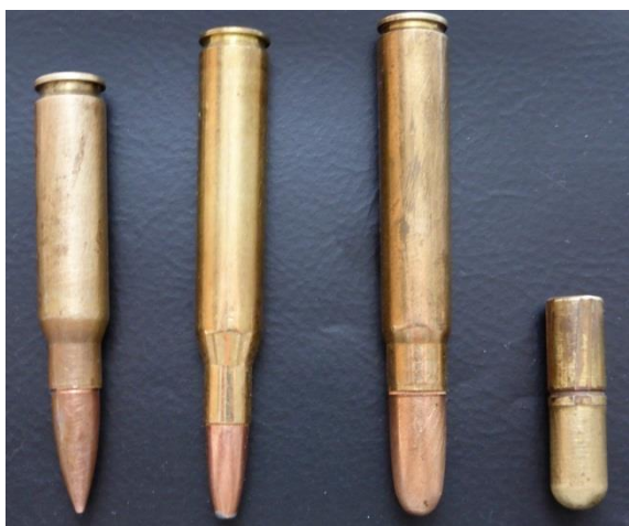
Fig. 5. The figure shows different types of bullets. From the left: pointed, full metal jacket calibre .308, soft nosed calibre .30-06, round nose, full metal jacket calibre 9.3, and round nose, full metal jacket calibre .375. Photo: EO Øen.
