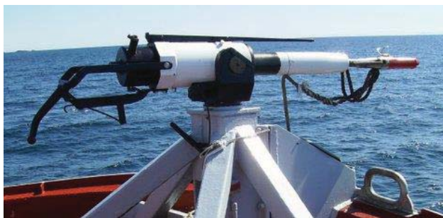
50mm Kongsberg whaling gun with harpoon and penthrate grenade.
